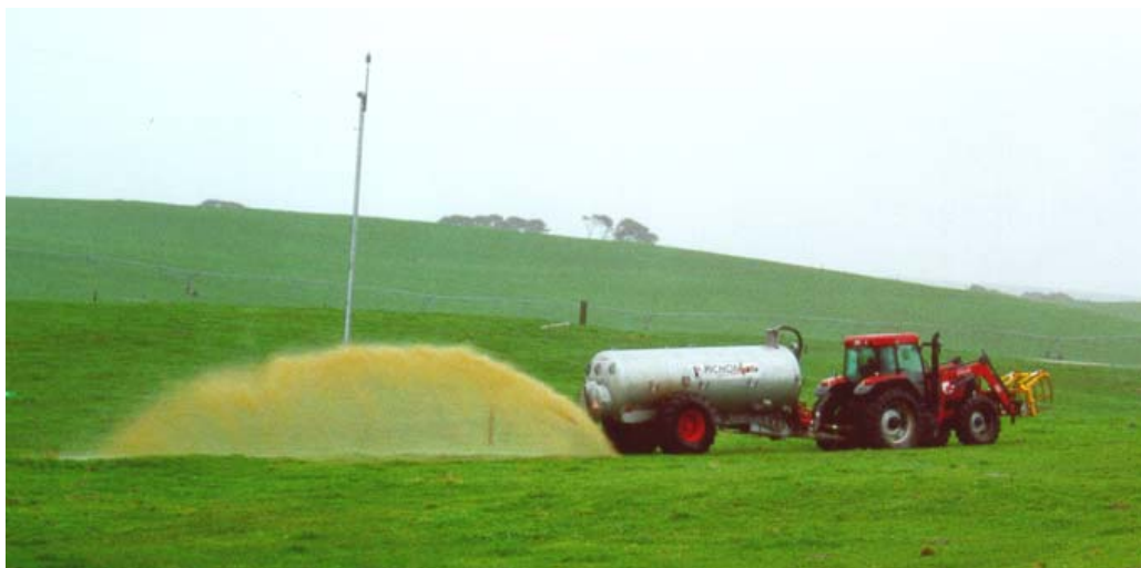
Spreading effluent using a slurry tanker fitted with a splash plate spreading system
